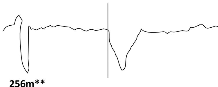
PVFO . 54\* Note: railway signalling cable is normally 54, but always check.
