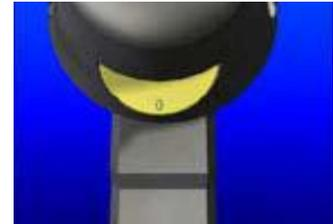
**IMPORTANT!** The normal lift height is 2mm (setting 0) this is very important for the arc and energy amount. Too high lift height will increase the risk of a "cold brazing", too low lift height will reduce the time and increase misfires.
