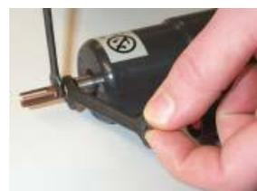
5. **Never twist the shaft when mounting the pin holder.**
