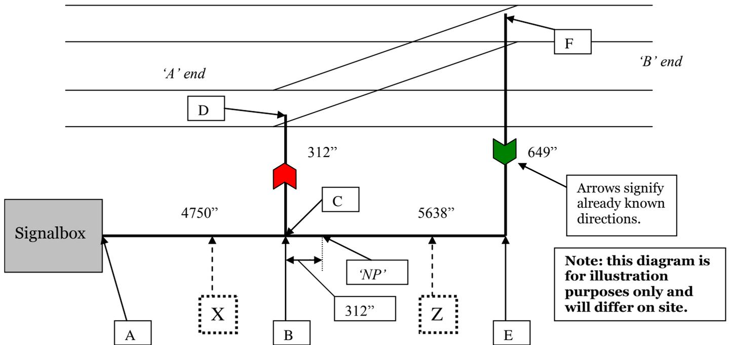
The working out should be done in two halves; the signalbox end first between A & D, (the rodding in the signalbox is disregarded as this is in a cool place and not subject to direct sunlight so is not affected by temperature changes). After this is done the second part is worked out from B to F, also using part of the first end (C-D).
